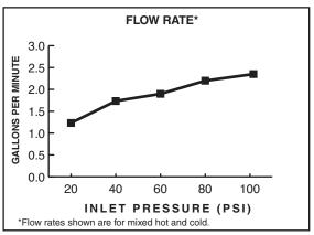
2.2gpm/8.3L/min. FLOW RATE
