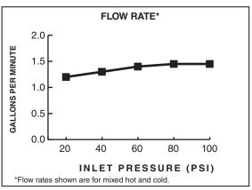
1.5gpm/5.7 L/min. FLOW RATE
