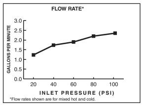
2.2gpm/8.3L/min. FLOW RATE
