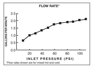
1.8gpm/6.8L/min. FLOW RATE
