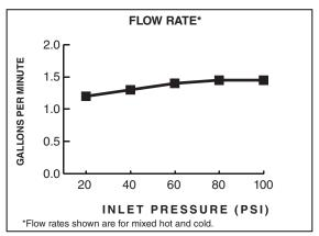
1.5gpm/5.7 L/min. FLOW RATE
