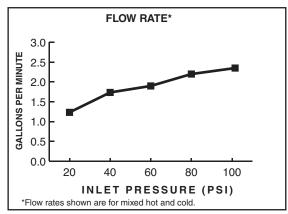
2.2gpm/8.3L/min. FLOW RATE
